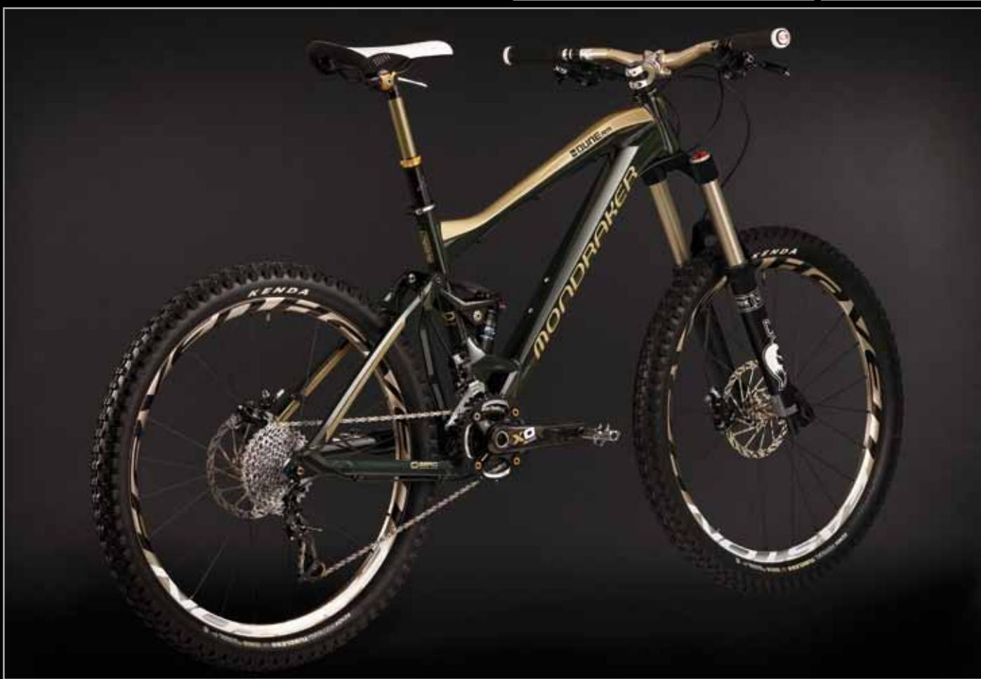
The Dune's are upgraded with a new frame with an important emphasis on the new Stealth (Side Alloy Structure) rear triangle. Thanks to this new detail and to the new fork Fox 36 the new Dune weights 400 grams less than its predecessor.
