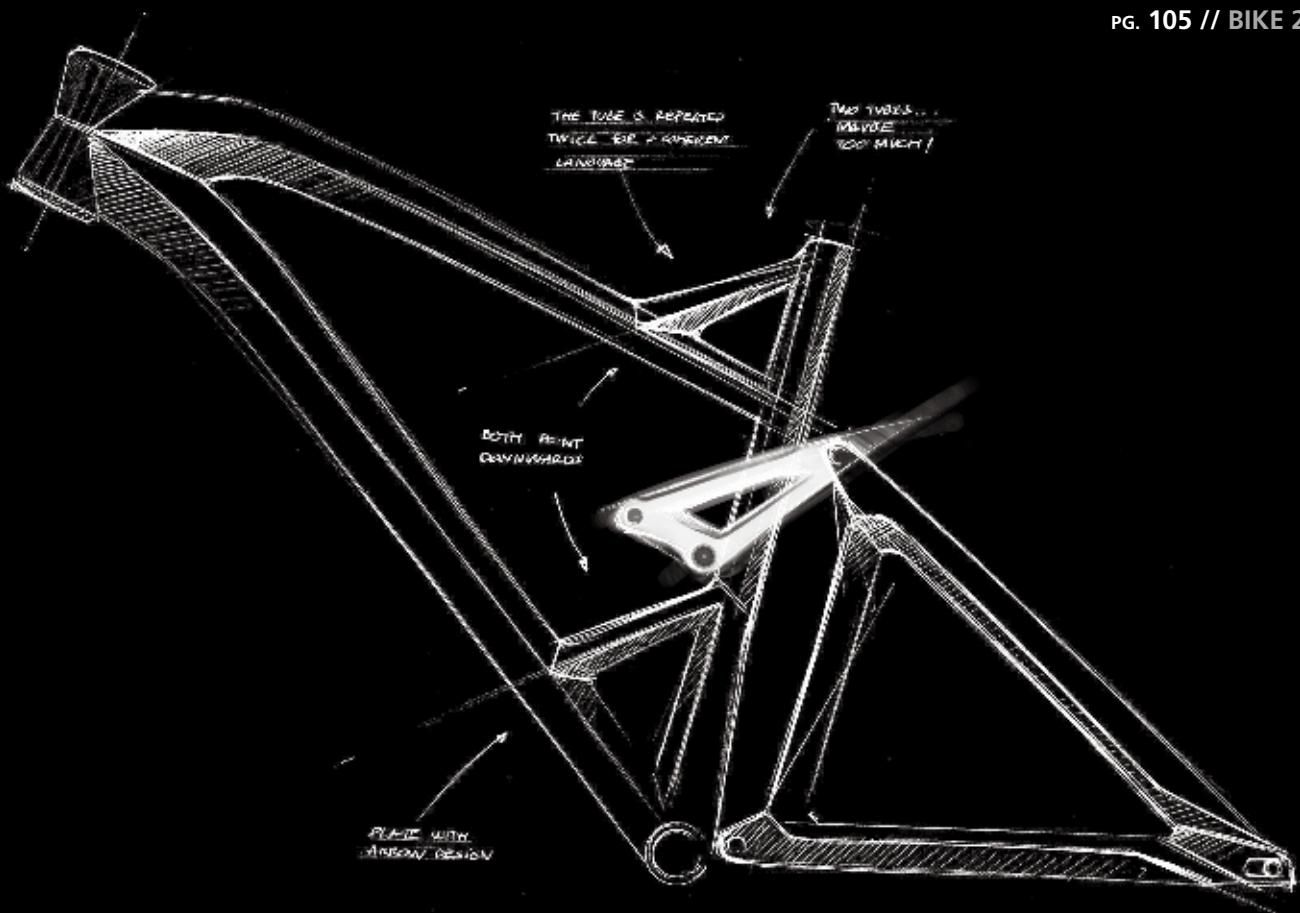
The Stealth technology is completely new, characterised by the rectangular shapes used in manufacturing as opposed to the more traditional round tubes. Each tube is carefully designed to carry out a specific function. By optimizing the production process, selecting the best materials, using tapered tubing and a selection of different alloys we can create an ultra-light tube set that is more resistant and rigid in the high stress areas of the frame.
