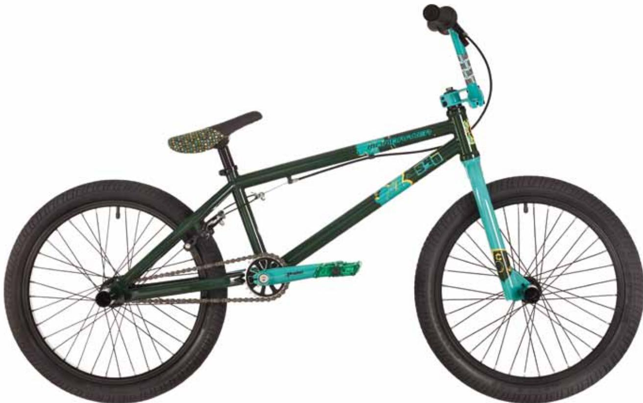
New frame and new geometry on all models because of a shorter chainstay and seat tube. This year the models 360° and 180° inherit specs of their older sister like for instance the new stem Abyss Indy, U-brake and the pivotal saddle system, all this to make them look even cooler.
