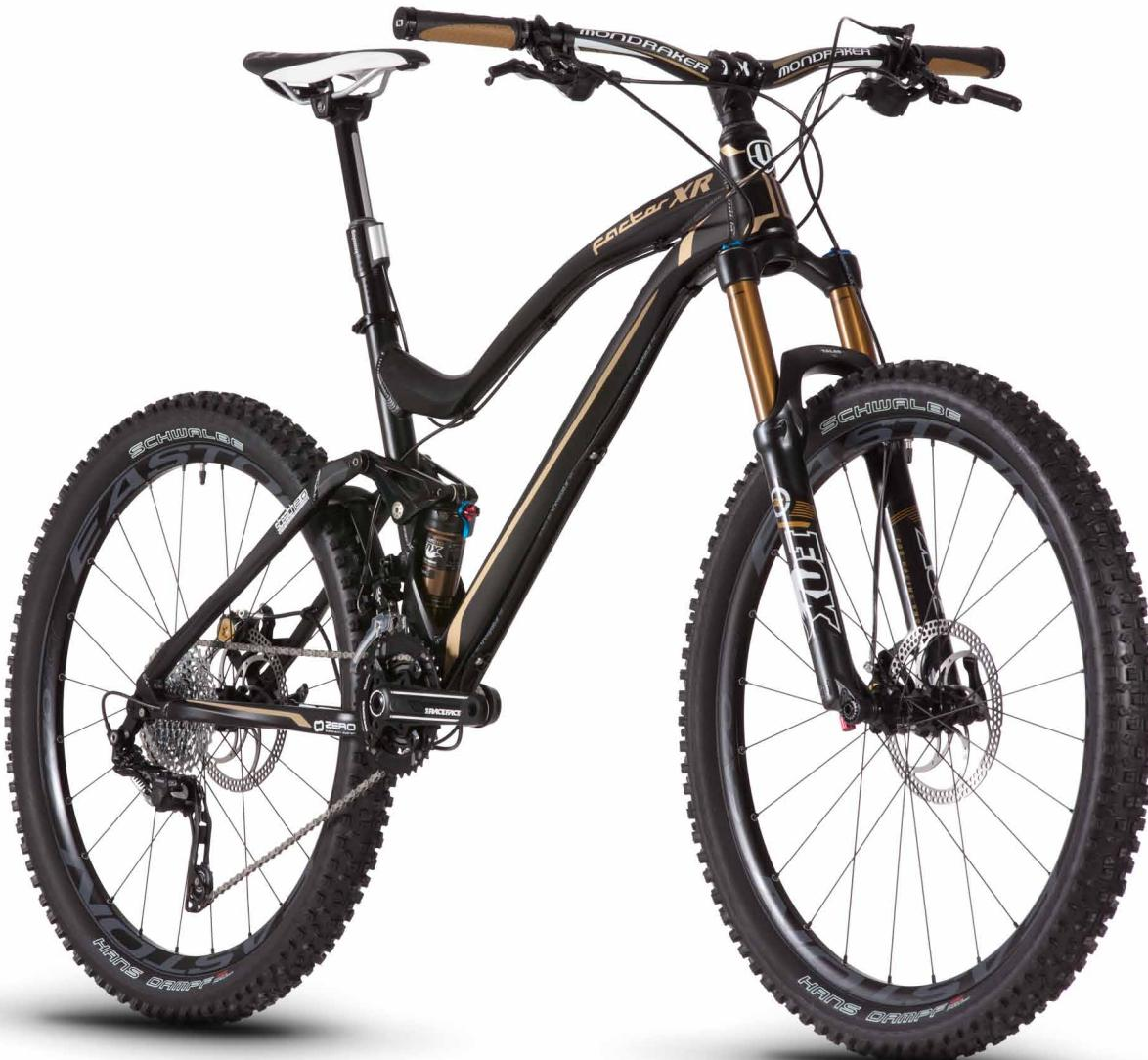
The Forward Geometry is compatible for all kinds of bikes and riders. So proves the Factor XR with its 120mm rear travel and a 400g lighter weighing frame compared to last year thanks to Stealth 2.0 tubing.
