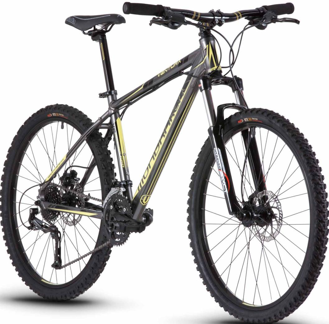
All the characteristics of the Ventura range offered to our female riders. An adapted geometry for female posture, a fork with softer compression, a shorter stem, a smaller handlebar, foam grips and a special specific saddle make this bike very comfortable during the ride.
