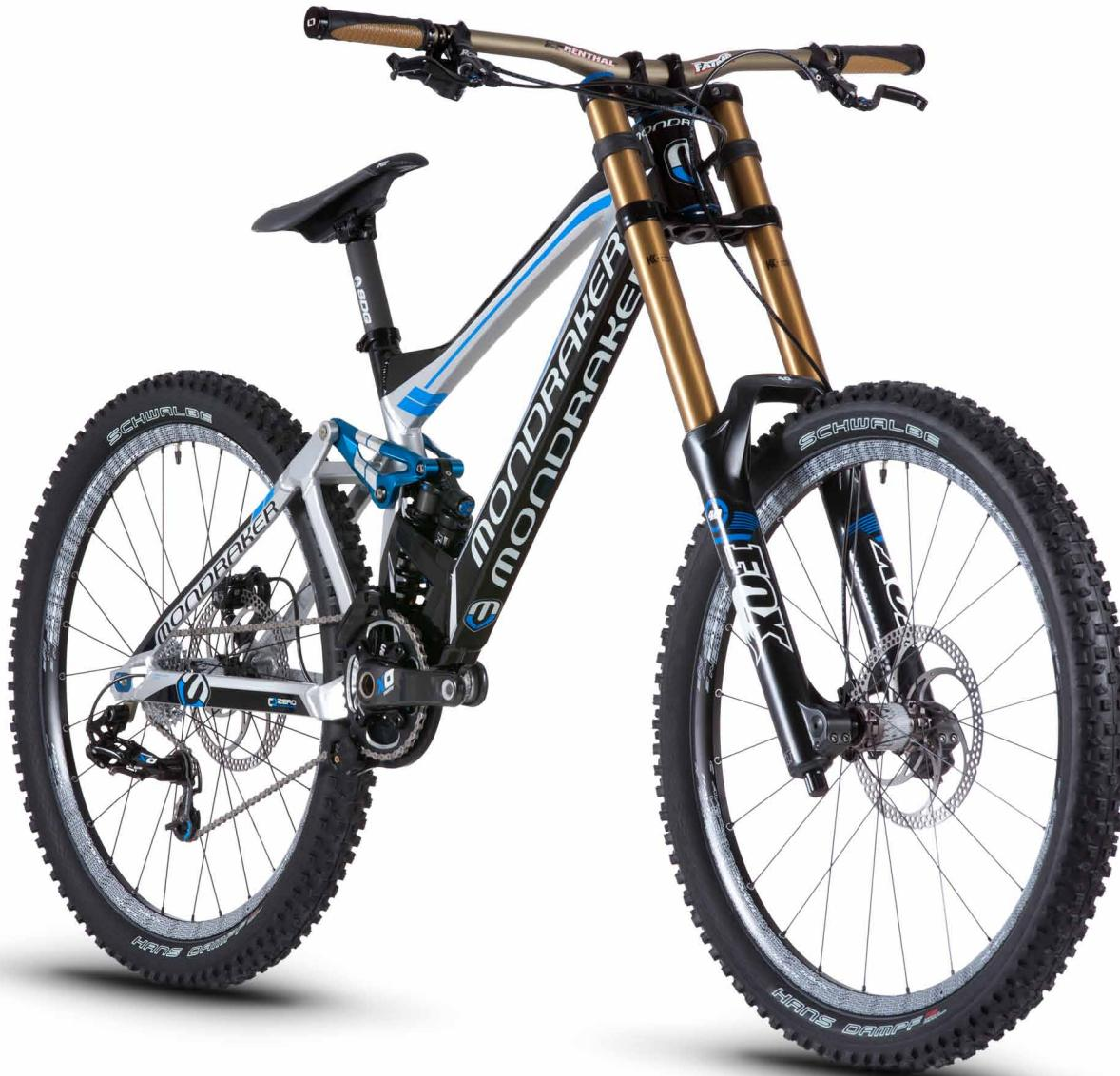
The new Summum frame has had an upgrade to offer an even better suspension performance thanks to the new kinematics and the use of bearings in the eyelets of the shock. This together with a new design of the rear triangle allows us to shave off 200g with which the Pro Team version slips underneath the 15kg.
