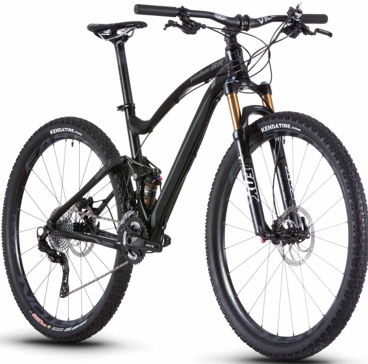
Zero Suspension applied on a 29er, a challenge that has exceeded all our expectations. The 110mm of travel together with a very compact geometry make the new Factor 29er an amazingly agile "mile shredder".
